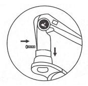
4. to haul down the stainless steel ring until the end of the hanging, make it connected with the crane boom, lastly fix them with the small bolt
