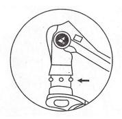
3. to oil four small steel balls, then plug them into the small round hole in the end of the
