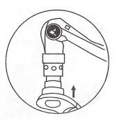
2. to insert the crane boom into the hanging, until joint completely.
