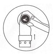
1. to telescope the stainless steel to the end of the hanging, and above the small round hole.
